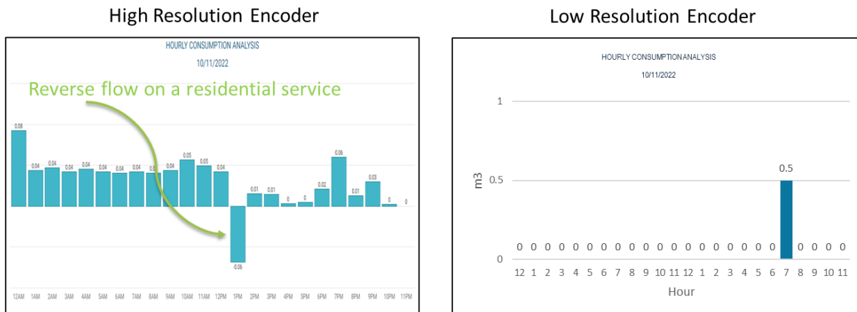
Exhibit 57: Reverse Flow - High vs Low Resolution Encoder Registers
