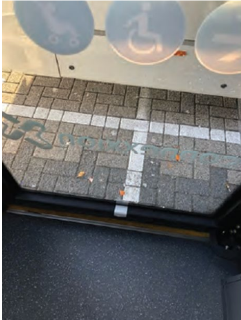
Figure 64. Example of alignment markers inside/outside the bus to help operators with positioning
