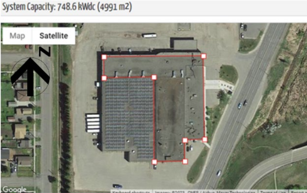
Figure 72. Fort Williams Rd Scenario 1 - Enclosed area shows the additional coverage of solar panels over the remaining building space.
