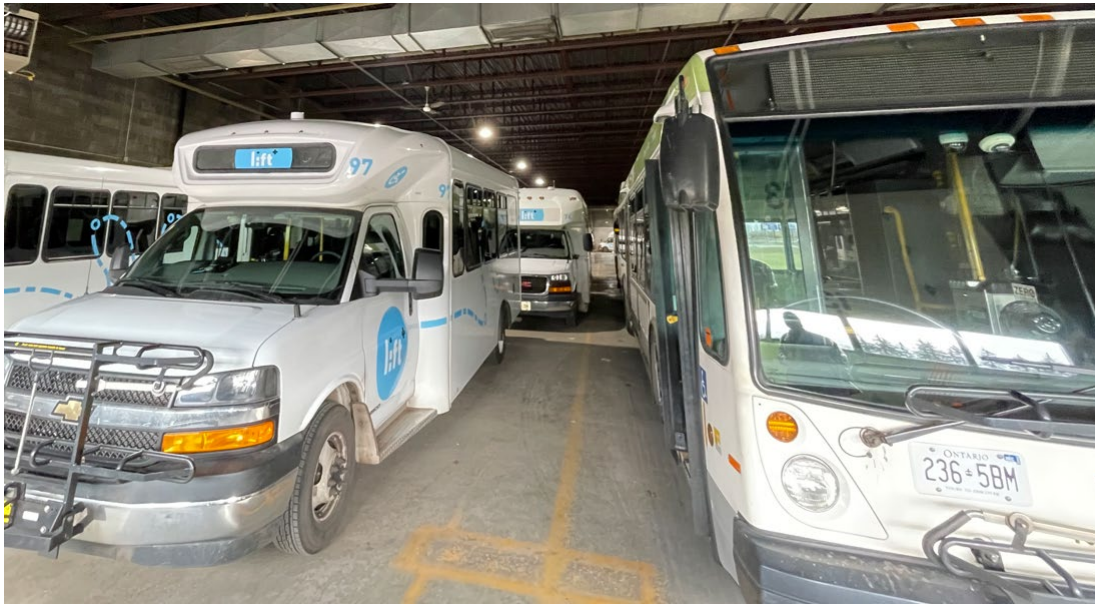
Figure 57. Limited space between vehicles at Fort William Road Transit Garage
