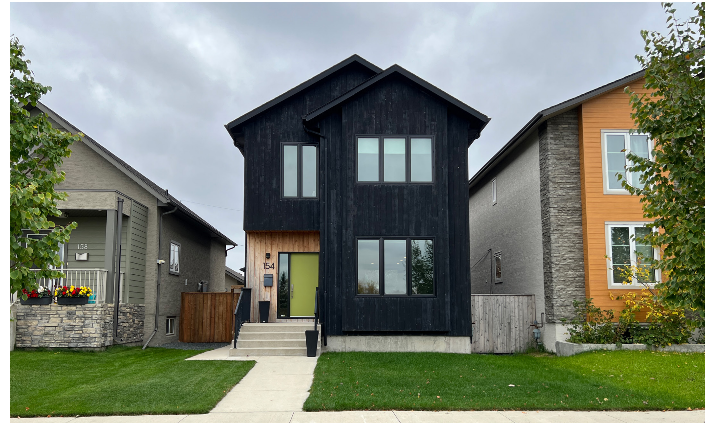
Front entry doors should incorporate a vision panel, with building elements projecting from the facade in the front yard encouraged to add visual interest.
